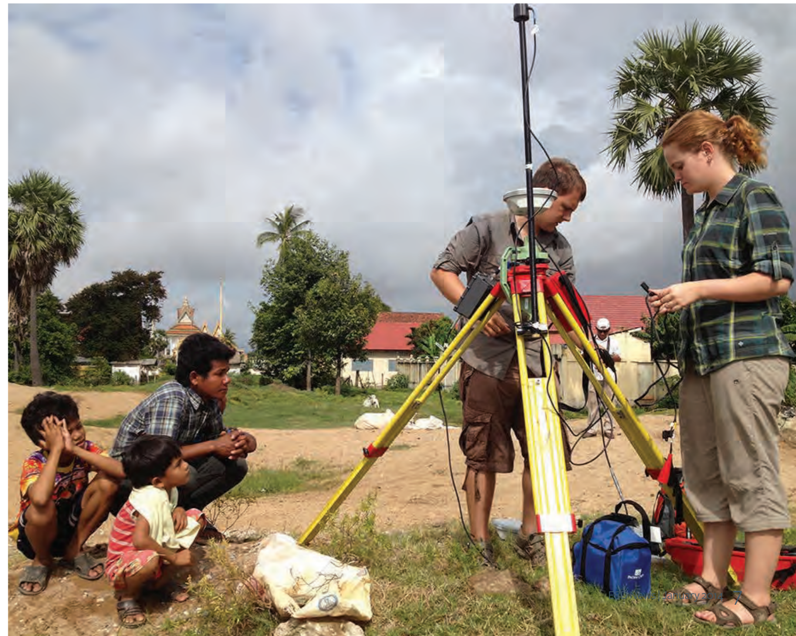
Setting up the dGPS basestation
